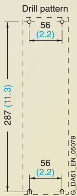
Fixing with M4 bolts
